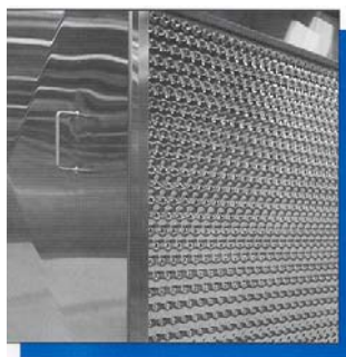
Figure 2-9. Falling film chiller showing vertical plates and a view of a plate
